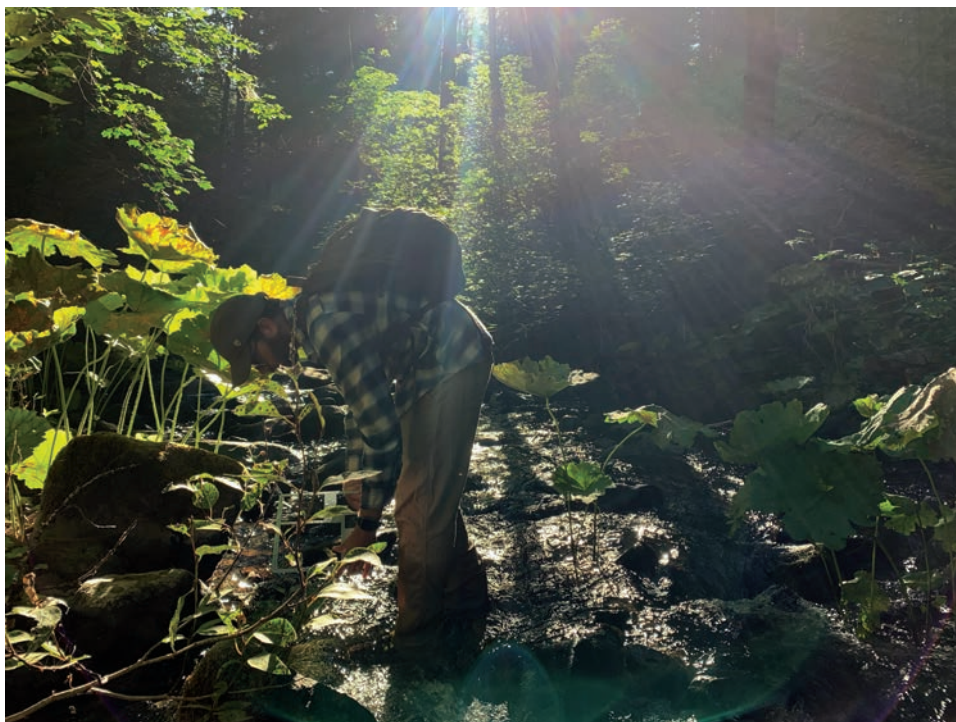
Chris Resinger (WRTC) uses a gravelometer to estimate the sizes of rock substrate in Corral Creek for a Stream Condition Inventory Survey
