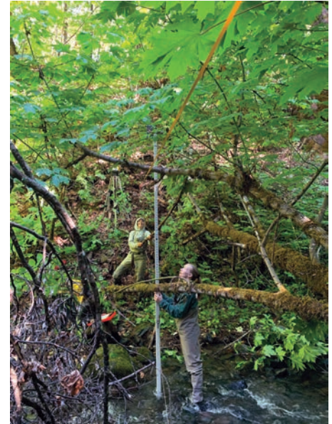
WSP Corpsmember Christine Burchinal and RCD staff Veronica Klenk move foliage out of the way to create a line of sight for the laser level in order to take cross-section measurements of Price Creek at permanent monuments of a Stream Condition Inventory Survey
