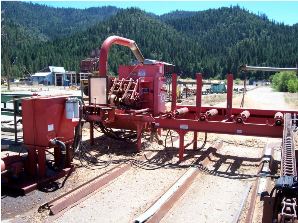
Figure 12: Small Diameter Utilization, post and pole peeler in Hayfork. Photo by Annette Hale, WRTC
