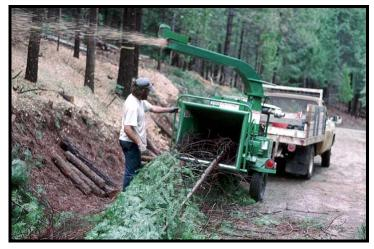
Chipper Being Used to Dispose of Trees from Fuels Reduction Project
