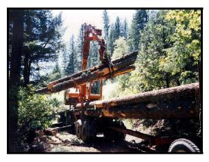
A heel boom loader is used to load logs on a narrow road, similar to roads found on the plan area. Specialized equipment such as this can be used to eliminate landings and reduce other impacts of logging.
